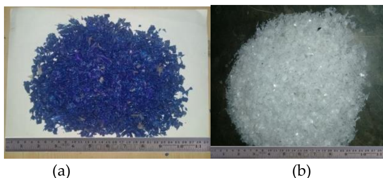
Figure 2: (a) Chopped/recycled HDPE (bottle cap) and (b) Pellets of LDPE (infusion bottle)
