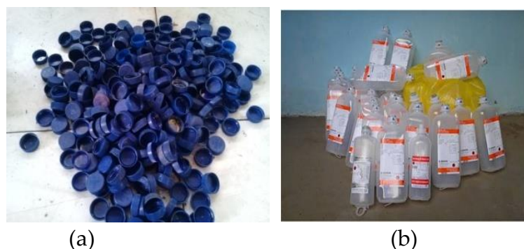
Figure 1: The raw materials: (a) HDPE (bottle cap) and (b) LDPE (infusion bottle)
