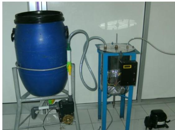
**Gambar 7. Foto *Sequencing Batch Bioreactor***
