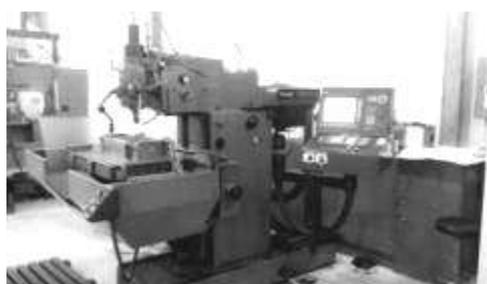
Gambar 2. Mesin Frais CNC Deckel FP4NC
