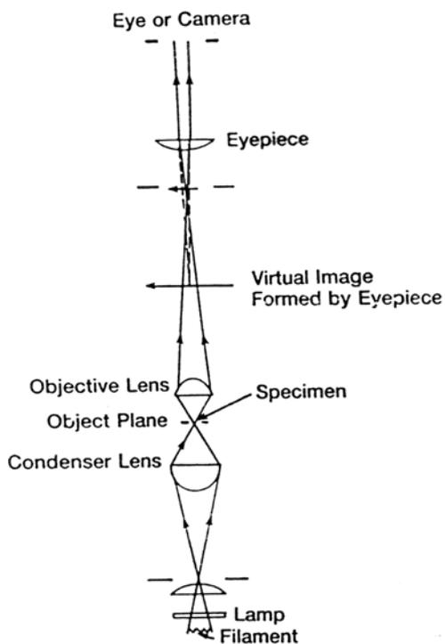
Gambar 1: Skema Mikroskop Optic (sumber Sibilia, J.P)
