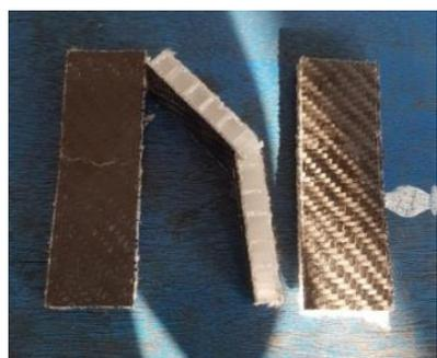
**Gambar 10. Patahan Komposit Karbon Sandwich Core Honeycomb 2 Lapisan Atas**
