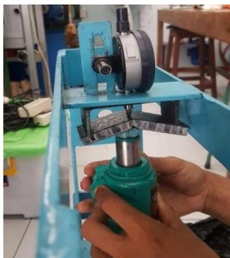
Gambar 7. Proses uji bending
