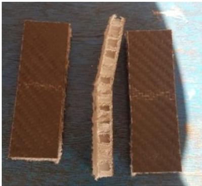
**Gambar 9. Patahan Komposit Karbon Sandwich Core Honeycomb 1 Lapisan Atas**
