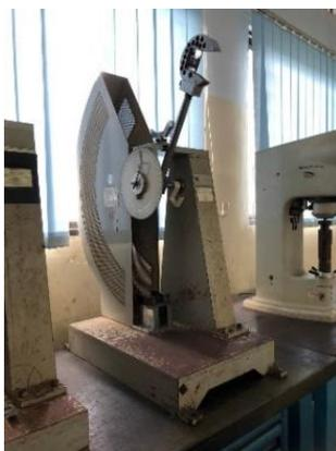
Gambar 4. Proses Uji Impact
