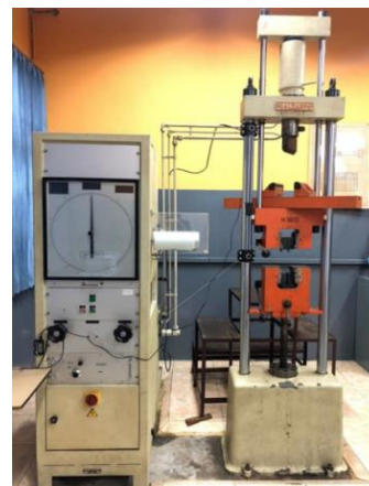
Gambar 2. Universal testing machine (UTM) Galdabini tipe PM10
