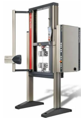
Gambar 4. Universal Testing Machine merk Zwick Roell
