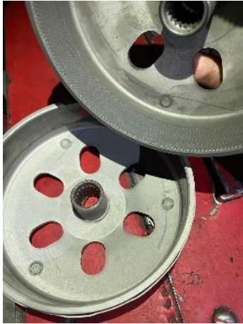
Gambar 3. Clutch housing bubut kartel
