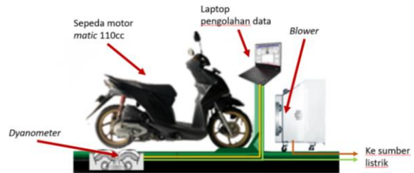
Gambar 6. Setting peralatan dyno test
