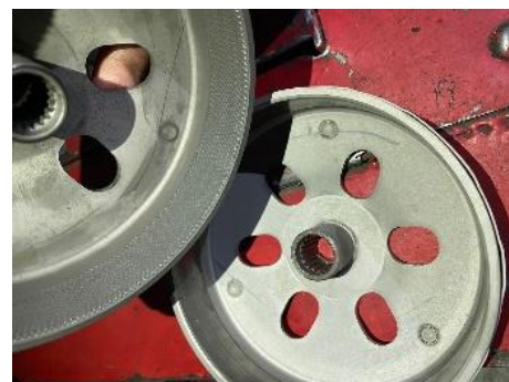
Gambar 3. Clutch housing bubut kartel
