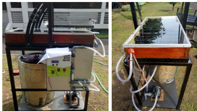
Gambar 3. Pengujian Solar Water Heater
