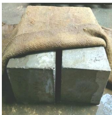
Gambar 4. Proses Curing Beton
