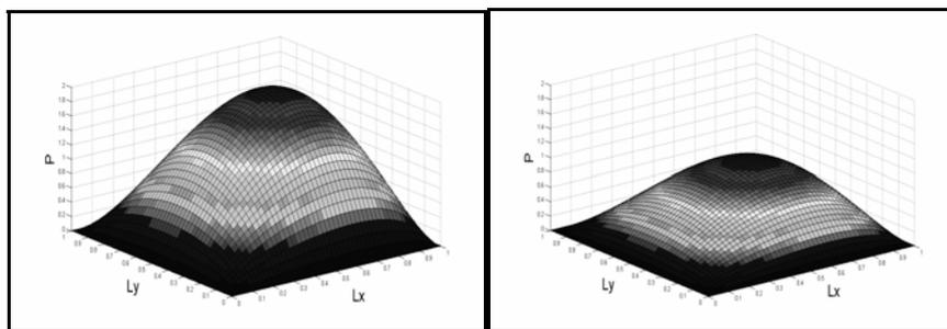
Fig. 4. Pressure distribution for (a) no-slip analysis, (b) slip boundary analysis
