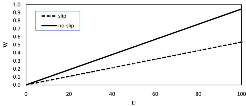
Fig. 5. Effect of the sliding velocity on the load carrying capacity
