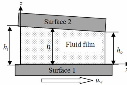
Fig. 2. Schematic of a sliding micro-gap with slip boundary
