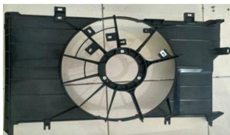
**Gambar 1. Tampak Depan *Shroud Fan Assy (No Hole)***
