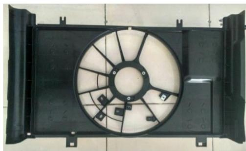
**Gambar 2. Tampak Belakang Shroud Fan Assy (No Hole)**
