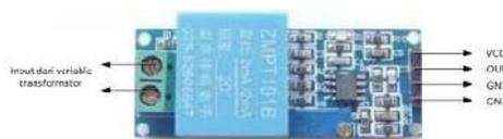
Gambar 4. Modul sensor tegangan ZMPT101B
