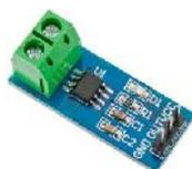
Gambar 3. Modul sensor arus ACS712
