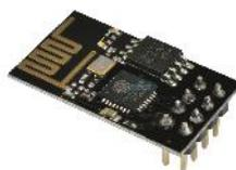
Gambar 5. Modul ESP8266-01
