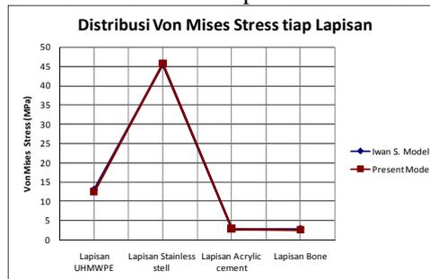
Gambar 4. Plot distribusi *von Mises stress* tiap lapisan
