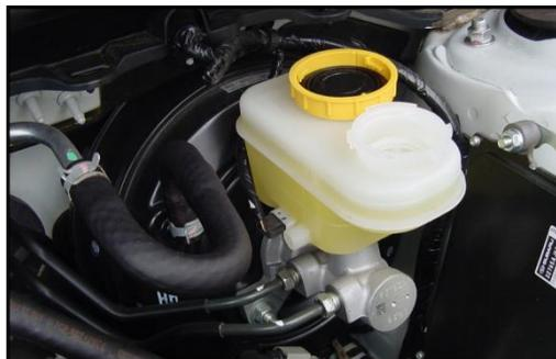
**Gambar 4 Sensor level brake fluid**
