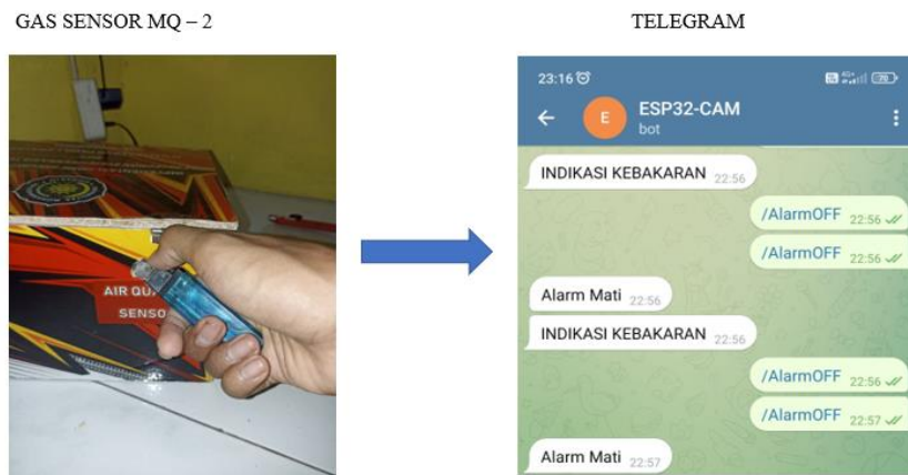
Gambar 4. Pengujian sensor Gas MQ – 2
