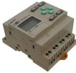
Gambar 1. PLC OMRON TYPE ZEN 10 I/O
