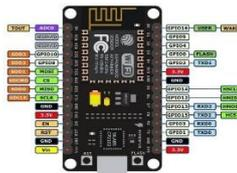
Gambar 1.1 NodeMCU ESP8266 (<https://www.nyebarilmu.com/>)
