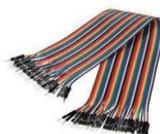
**Gambar 1.9 Kabel Jumper** (<https://www.arduinoindonesia.id>)
