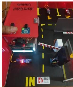
Gambar 3.5 Pengujian Sensor TTP223B
