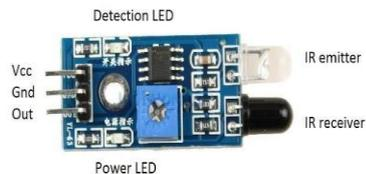
Gambar 1.4 Sensor Infrared (<https://dosenit.com/>)
