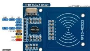
Gambar 1.6 Module RFID (Immersa-Lab, 2018)
